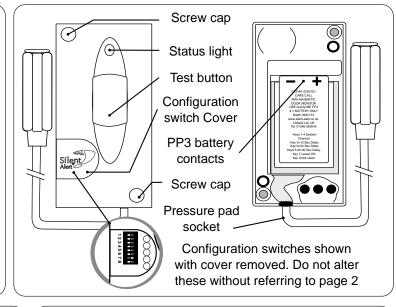
2. Install a 9 volt PP3 alkaline or lithium battery making sure to observe the correct polarity.
